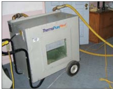
Areas of the ranch style home were treated with heat to control bed bugs.
